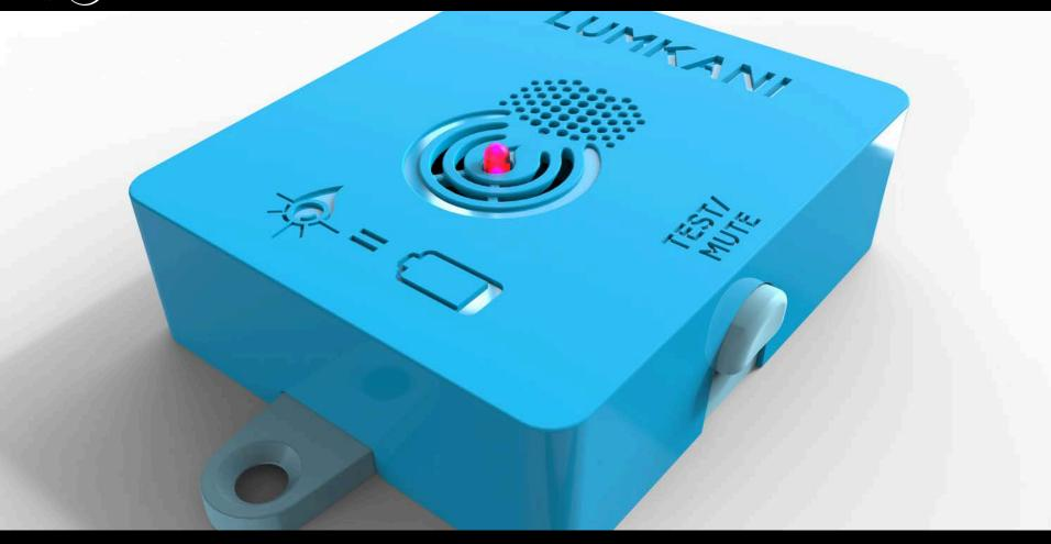
In January 2013, a series of fires hit two Cape Town townships, leaving 4,000 homeless. Launched later that year, Lumkani is a low-cost smart fire detector that can distinguish between heat from cooking and a dangerous fire. Simple radio frequency technology means that if a fire is detected by one device, all others in a 100-meter radius will also sound an alarm.
